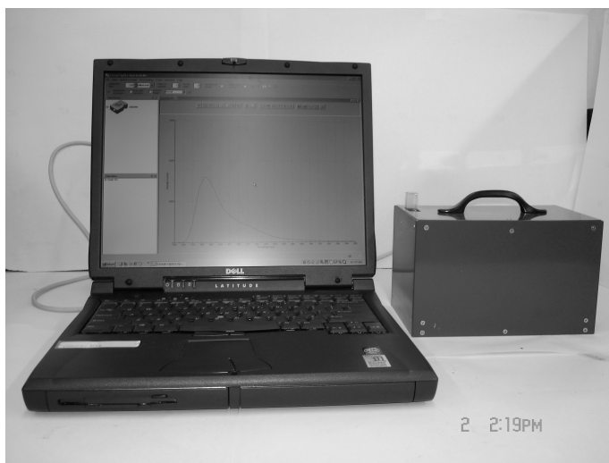
Figure 6: Photograph of the minimized NSET probe box, connected with laptop computer for data acquisition
